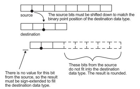
As the diagram shows, the source bits are shifted down so that the binary point matches the destination binary point position. There is no value for the highest bit from the source, so sign extension is used to fill the integer portion of the destination data type. The bottom five bits of the source do not fit into the fraction length of the destination. Therefore, precision can be lost as the result is rounded.
